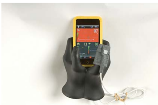
The Phone Oximeter: A prototype of the first cell phone-based pulse oximeter.
