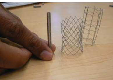
Compare the heights of the three stents: before expansion (left); stent with a diamond geometry which shrinks in height as it is expanded (middle); a stent geometry does not shrink after it is expanded (right).
